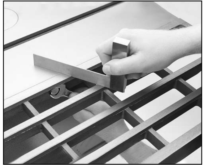
Figure 23. Checking table to wing alignment.
